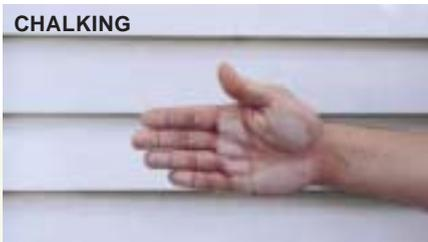
**Excessive Chalking** is the release of an unacceptable amount of pigment as a fine powder on the surface of the paint. While some degree of chalking helps keep the surface clean, excessive chalking can result in serious color fading, rapid film erosion, and rundown over other surfaces. Among the causes of excessive chalking are:
