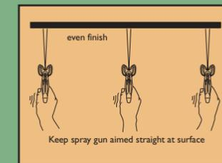
Also, start your stroke before you pull the trigger, and continue it after releasing the trigger. If you don't, there will be heavy spots of paint where you start and stop. Reverse your stroke direction and apply the return stroke in the same manner.
