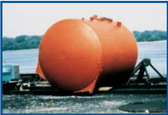
Tank after primer application.
